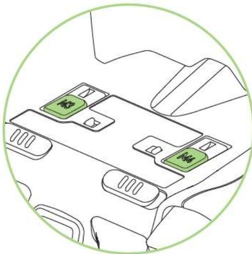
To open the trigger cover, simply pull aside the cover release switches.
