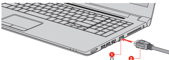
Figure 4-17 Connecting the RGB cable to the External RGB monitor port
