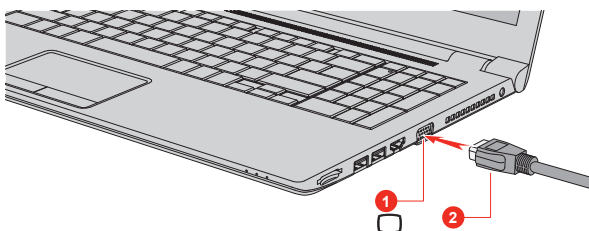
Figure 4-17 Connecting the RGB cable to the External RGB monitor port
