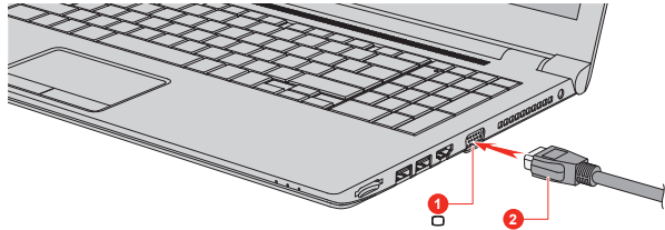
Figure 4-16 Connecting the RGB cable to the External RGB monitor port
