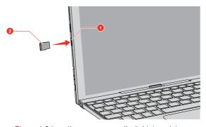
Figure 4-6 Inserting memory media (tablet mode)
