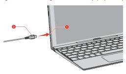
Figure 4-8 Connecting the HDMI cable (tablet mode)
