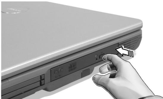
When the power is off, you can eject the drive tray using the emergency eject hole. See page 60.
