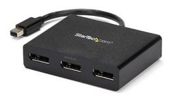
This MST hub lets you connect three DisplayPort monitors to your Mini DisplayPort computer. MST works on any Windows device that supports DisplayPort 1.2, such as models of the Lenovo Think Pad and Microsoft Surface. When connected to earlier revisions of DisplayPort, such as DP 1.1 the MST hub acts as a video splitter.
