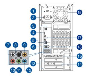
**Voltage selector switch.** Switch to select the appropriate system input voltage.
