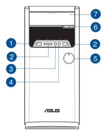
**USB 3.0 ports.** These Universal Serial Bus 3.0 (USB 3.0) ports connect to USB 3.0 devices such as a mouse, printer, scanner, camera, PDA, and others.
