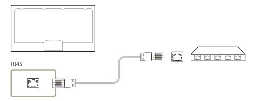
• Use Cat7(\*STP Type) cable for the connection. \*Shielded Twist Pair
