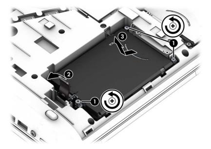
7. Lift the hard drive (3), and then pull the hard drive out of the hard drive bay.
