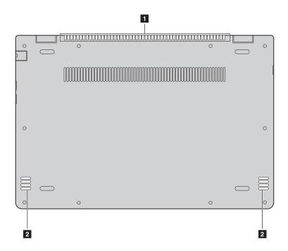
1 Ventilation slots Dissipate internal heat.
