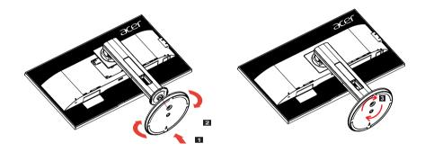
Remove: Reverse the steps to remove the base.
