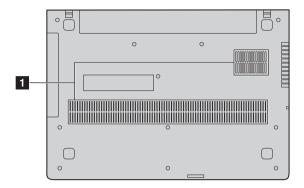
**Ventilation slots** Allow air to enter the computer for cooling.
