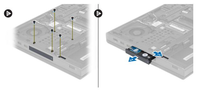
4. Flex the hard-drive bracket outward and pull out the hard drive from the bracket.
