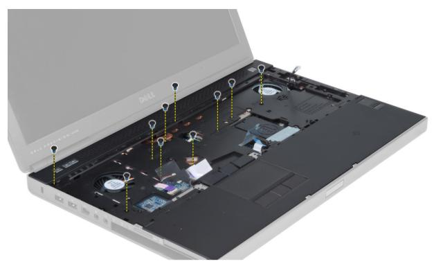
12. Lift the left edge of the palmrest. Release the tabs on the right edge of the palmrest and remove the palmrest from the computer.
