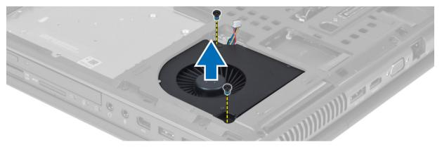
4. Disconnect the processor-fan cable.
