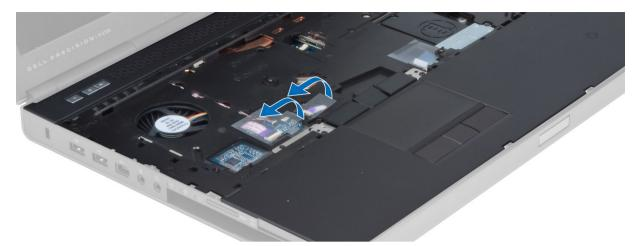
$\textbf{7.} \hspace{0.5cm} \textbf{Disconnect the media board cable and the speaker cable from the system board.} \\$
