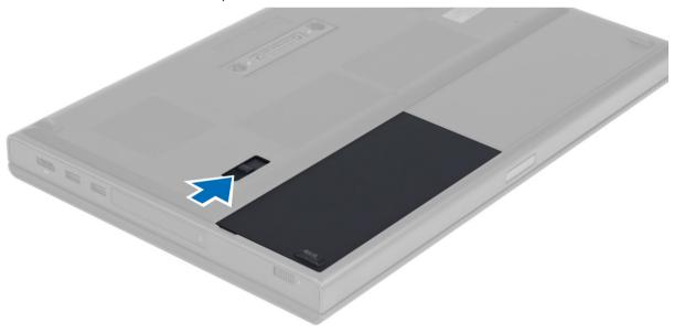
3. Lift and remove the battery from the computer.
