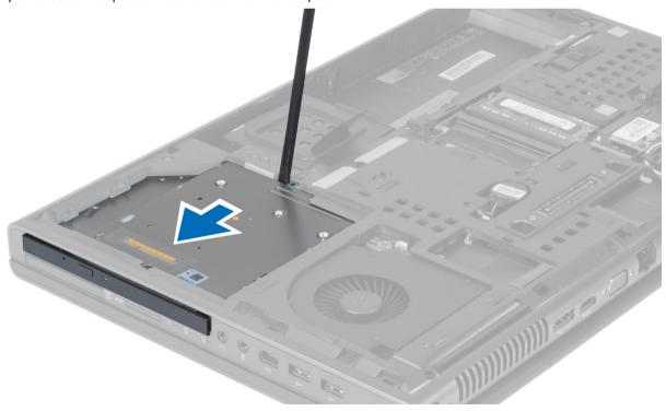
5. Remove the screws that secure the drive-latch bracket to the optical drive and remove the bracket.
