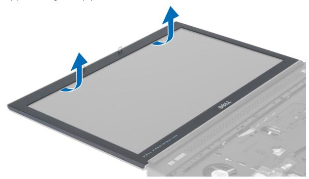
**4.** Work your way around the sides and top edge of the display bezel and remove the display bezel from the computer .
