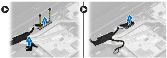
Remove the screws that secure the display assembly to the computer. Remove the display assembly from the computer.
