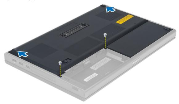
4. Lift and remove the base cover from the computer.
