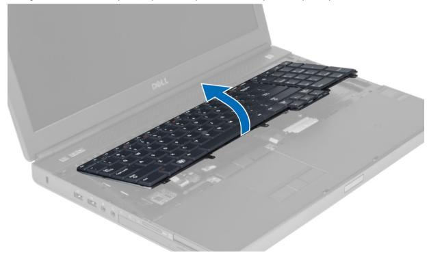
**5.** Disconnect the keyboard-data cable from the system board and remove the keyboard.
