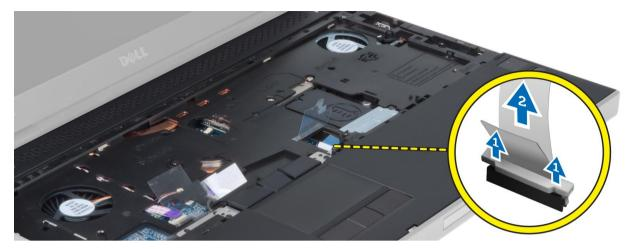
10. Disconnect the power button cable from the system board.
