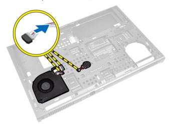
**4.** Disconnect the power connector cable. Remove the screws that secure the system board to the computer and lift the bottom edge of the system board at a 20–degree angle.
