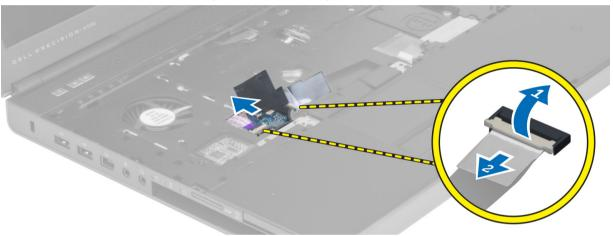
8. Peel the adhesive tape that secures the touchpad cable to the palmrest.
