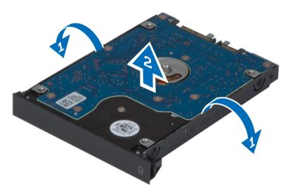
**NOTE:** A rubber filler is installed to the hard-drive bracket for 7 mm hard drives. It is designed to prevent vibrations and for correct installation of the 7 mm hard drives. 9 mm hard drives do not require the filler when installed into the hard-drive bracket.
