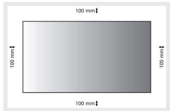
Allow adequate ventilation or provide air conditioning around the monitor, so that heat can properly dissipate away from the unit and mounting apparatus; especially when you use monitors in multiple screen.
