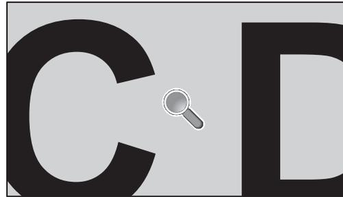
Using “SET/POINT ZOOM” button on a remote control allows to enlarge a partial of image. Press CH+/- button to zoom up or down. The image can be expanded from 1 to 10 times.
