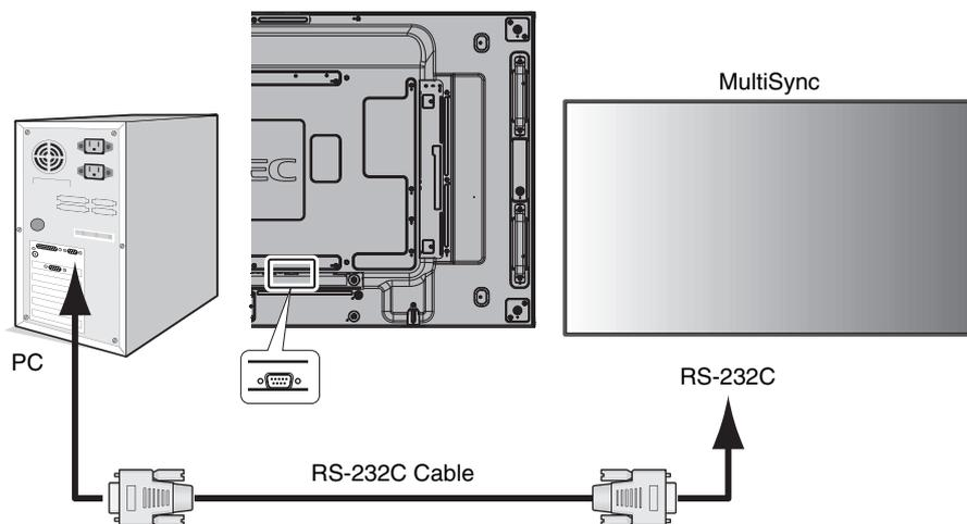
**NOTE:** If your PC is equipped only with a 25-pin serial port connector, a 25-pin serial port adapter is required. Contact your dealer for details.
