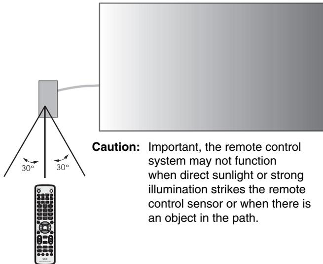
**Caution:** Important, the remote control system may not function when direct sunlight or strong illumination strikes the remote control sensor or when there is an object in the path.
