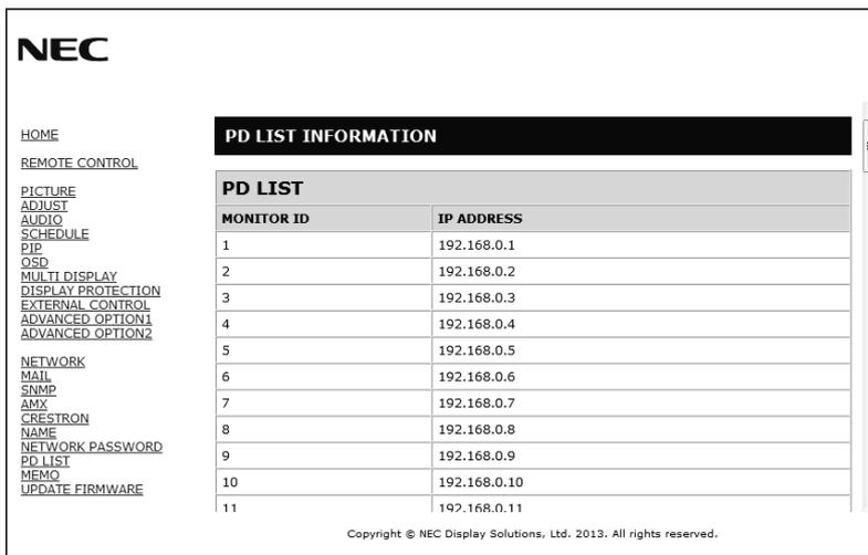
Show the list of ID and IP address of multiple monitors that are daisy-chained.
