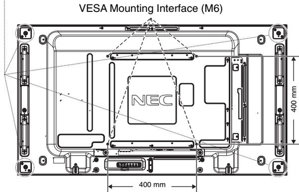
Mounting accessories can be attached with the monitor in the face down position. To avoid damaging the screen face, place the protective sheet on the table underneath the LCD. The protective sheet was wrapped around the LCD in the original packaging. Make sure there is nothing on the table that can damage the monitor.
