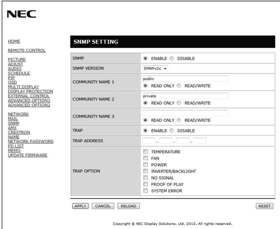
This function allows for getting status and controlling of a monitor via the network.
