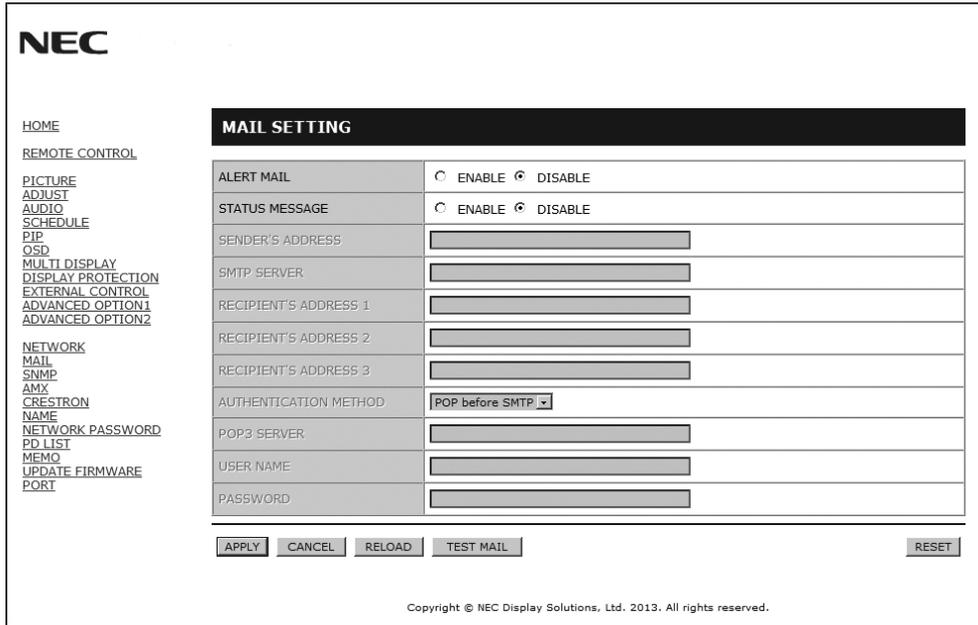
This option notifies your computer of an error message via e-mail when using wired LAN. An error message notification will be sent when an error occurs in the monitor.
