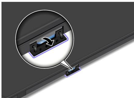
4. If a SIM card is preinstalled in the slot, push the SIM card inward a little, the SIM card pops out. Gently slide the SIM card out of the slot.
