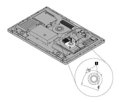
Figure 44. Removing the GPU fan
