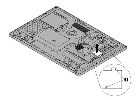
Figure 42. Removing the card reader
