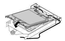
Figure 58. Installing the microprocessor socket cover
