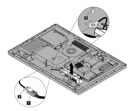
Figure 27. Removing the rear I/O assembly
