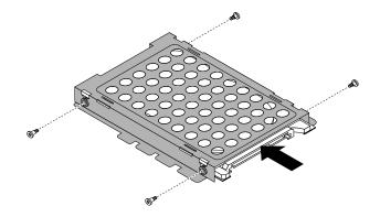
Figure 16. Installing the hard disk drive into the hard disk drive bracket
