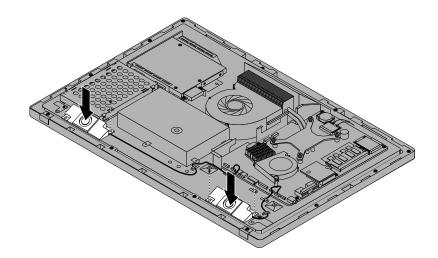
Figure 53. Installing the internal speakers
