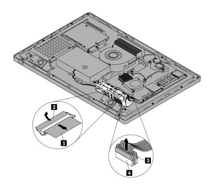
Figure 26. Disconnecting the HDMI and USB cables
