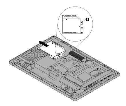
Figure 18. Removing the optical drive
