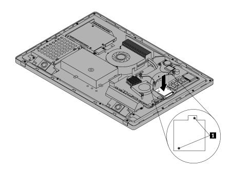
Figure 43. Installing the card reader
