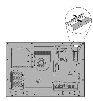
Figure 64. Connecting the LCD panel cable to the system board
