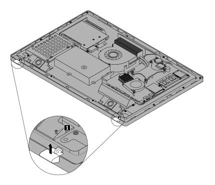
Figure 12. Removing the feet
