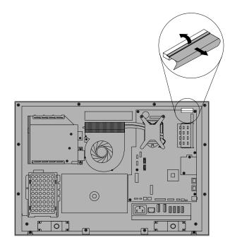
Figure 59. Disconnecting the LCD panel cable from the system board
