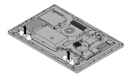
Figure 52. Removing the internal speakers
