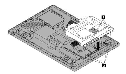
Figure 21. Positioning the system board shield onto the chassis
