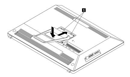
Figure 6. Installing the frame stand
