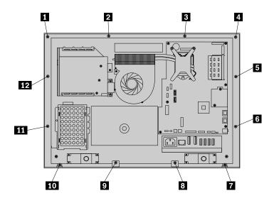
Figure 63. Installing the 12 screws to secure the bracket frame to the main bracket
