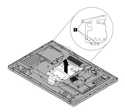
Figure 23. Removing the VESA mount bracket
