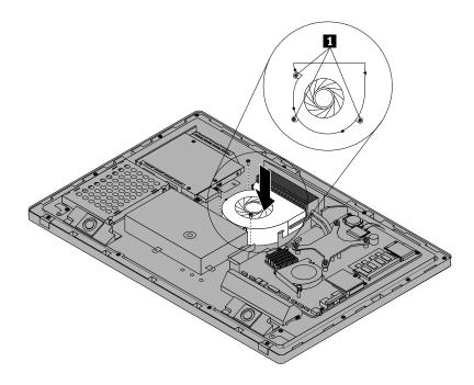
Figure 36. Installing the microprocessor fan
