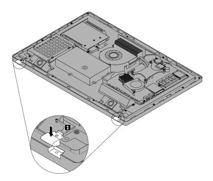
Figure 13. Installing the feet
