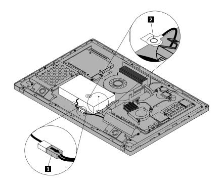
Figure 31. Disconnecting the power cable and earth wire
