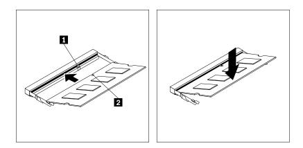
Figure 51. Installing a memory module
