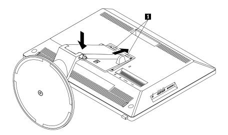
Figure 10. Installing the transformer stand
