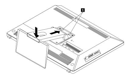
Figure 8. Installing the monitor stand
