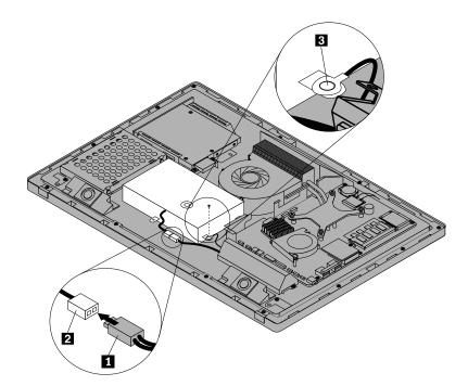
Figure 34. Connecting the power cables and securing the earth wire
