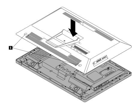
Figure 71. Installing the computer cover
