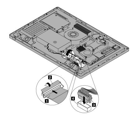
Figure 29. Connecting the HDMI and USB cables
