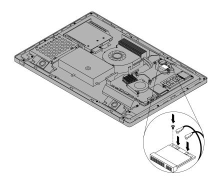
Figure 68. Securing the Wi-Fi card and connecting cables
