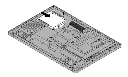
Figure 19. Installing the optical drive
