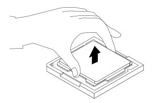
Figure 40. Removing the microprocessor
