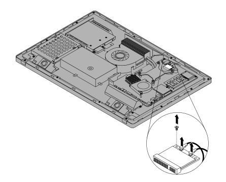
Figure 65. Disconnecting cables and removing the screw from the Wi-Fi card
