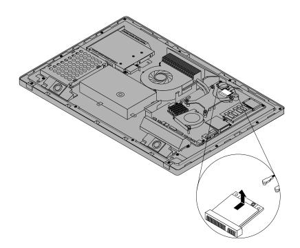
Figure 66. Removing the Wi-Fi card
