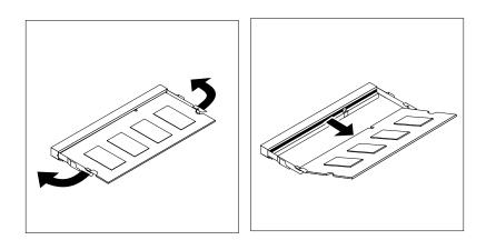
Figure 50. Removing a memory module
