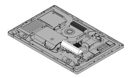
Figure 30. Installing the rear I/O assembly
