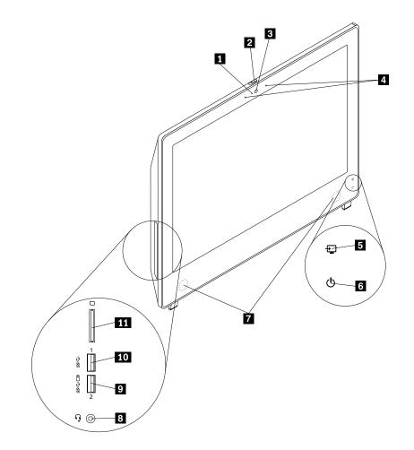
Figure 1. Front connector, control, and indicator locations
