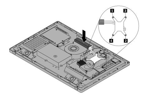
Figure 38. Tightening the four screws to secure the heat sink assembly
