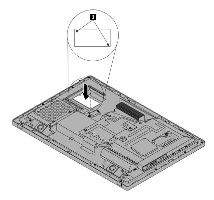
Figure 49. Installing the converter board
