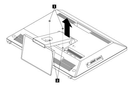
Figure 7. Removing the monitor stand
