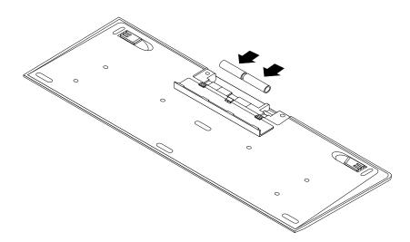
Figure 70. Installing the keyboard batteries
