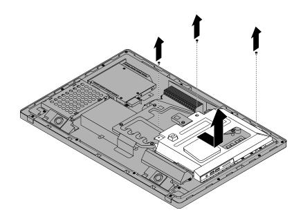
Figure 20. Removing the system board shield
