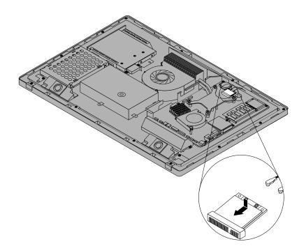
Figure 67. Installing the Wi-Fi card
