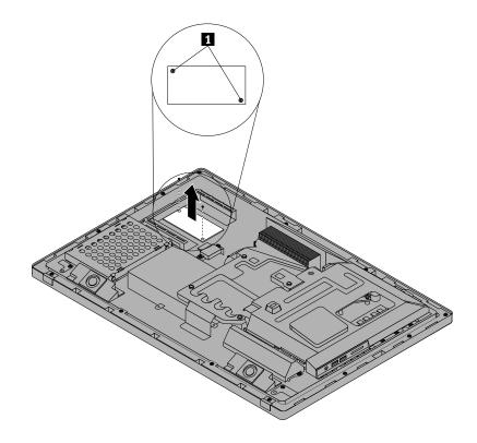
Figure 48. Removing the converter board
