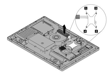
Figure 37. Loosening the four screws that secure the heat sink assembly
