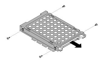
Figure 15. Removing the hard disk drive from the hard disk drive bracket
