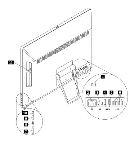
Figure 2. Rear connector locations
