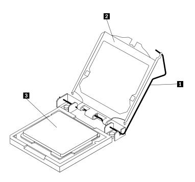
Figure 39. Accessing the microprocessor
