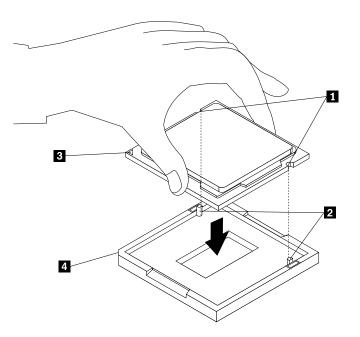
Figure 41. Installing the microprocessor
