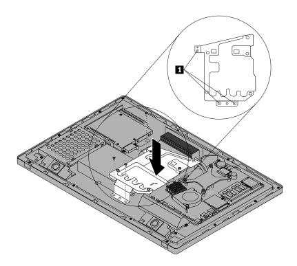
Figure 24. Installing the VESA mount bracket
