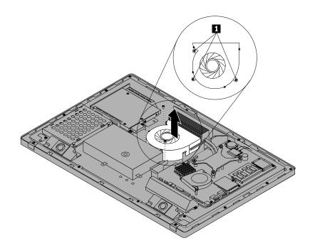
Figure 35. Removing the microprocessor fan
