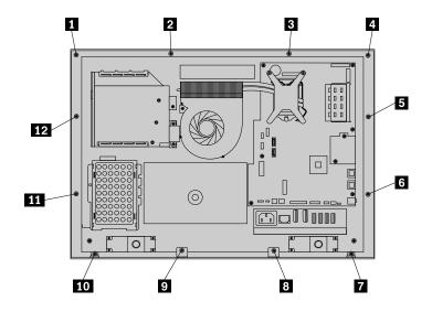
Figure 60. Removing the 12 screws that secure the bracket frame to the main bracket
