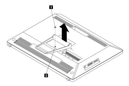
Figure 5. Removing the frame stand
