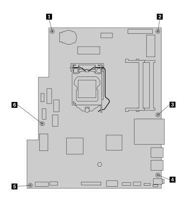
Figure 56. Removing the six screws that secure the system board
