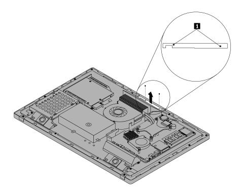
Figure 54. Removing the integrated camera
