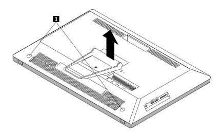
Figure 11. Removing the computer cover
