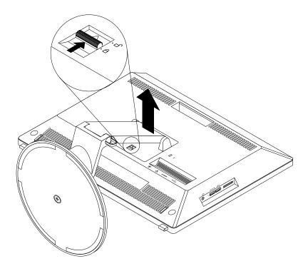
Figure 9. Removing the transformer stand
