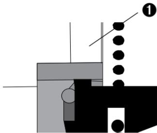
7. Adjust the right tractor to centre the paper holes on the pins, and push back the lock lever.
