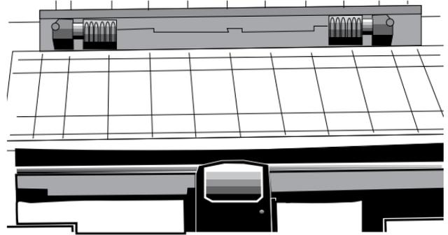
4. Move the right tractor over to fit the width of the paper.
