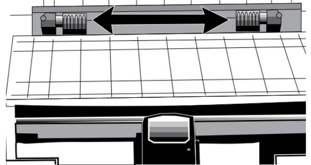
5. Place the first two holes in the paper over the tractor pins on either side and close the tractor covers.
