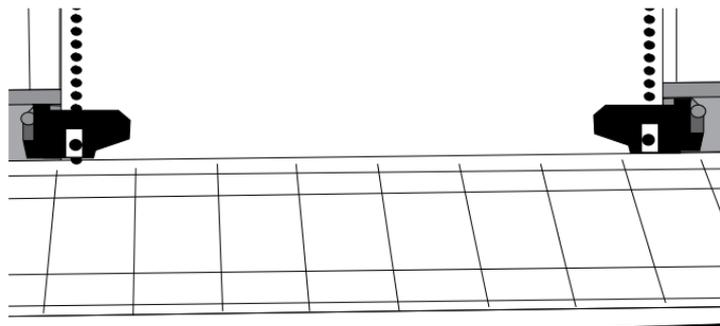
6. Move the left tractor to align the edge of the paper with the appropriate reference mark (❶), and push back the lock lever.
