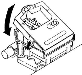
6. Turn the knob (1) in the direction of the arrow to take up any ribbon slack.
