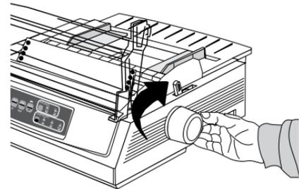
5. Remove the paper pieces, and use the platen knob to back the paper out.
