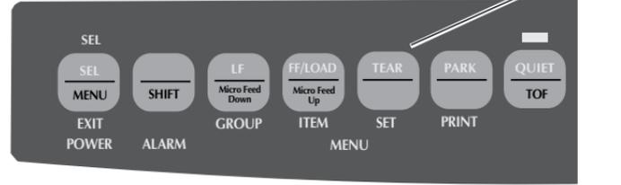
Use this feature to advance continuous-form paper up to the tear position by simply pressing **TEAR** (❶).
