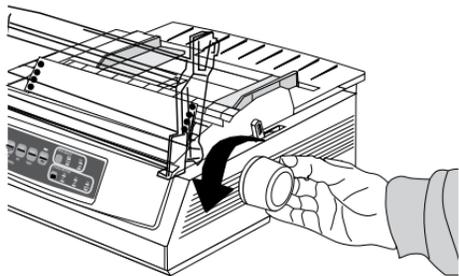
6. Swing the paper separator over, reload regular paper, and lower the paper separator back into place.
