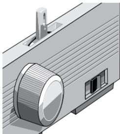
3. Open the carriage cover and lift the paper separator to the single-sheet position.
