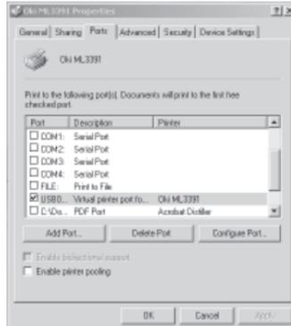
8. If the printer had formerly been used as a parallel or serial device and there is no output from the printer once a USB cable has been connected, check to see that the correct port has been selected. This information can also be found in the Properties folder but under the Ports tab. Amend as necessary.
