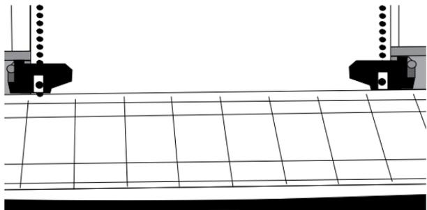
7. Replace the pull-up roller assembly, and close the access cover.
