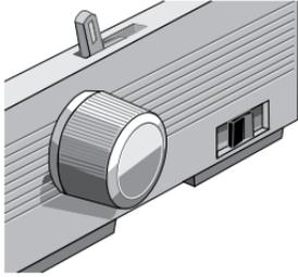
2. Grasp the paper separator, lift it slightly, pull back on it, then swing it forward.
