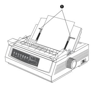
Note: The standard setting for the Top of Form (where the printing begins) is 2.54cm down from the top of the page. To change the setting, see the next column.
