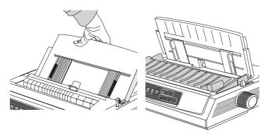
3. Pull up on the lock levers and open the tractor covers.
