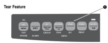
Use this feature to advance continuous-form paper up to the tear position by simply pressing **TEAR**  $(\mathbf{0})$ .
