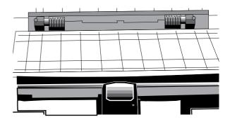
4. Move the right tractor over to fit the width of the paper.
