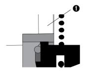
7. Adjust the right tractor to centre the paper holes on the pins, and push back the lock lever.
