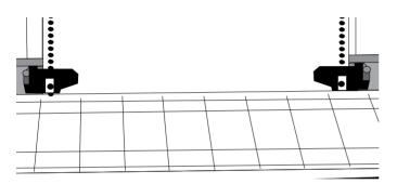
6. Move the left tractor to align the edge of the paper with the appropriate reference mark (**①**), and push back the lock lever.
