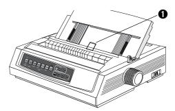
5. Adjust the paper feed guides (**1**) for the width of the paper and place a sheet of paper in the separator. The paper will feed into the printer.
