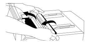
3. Use a clean, dry cloth to dust around the carriage shaft and platen. Remove any loose pieces of paper.
