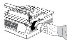
Swing the paper separator over, reload regular paper, and lower the paper separator back into place.
