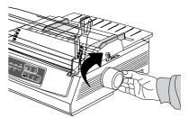
Remove the paper pieces, and use the platen knob to back 7. Replace the pull-up roller assembly, and close the access the paper out.
