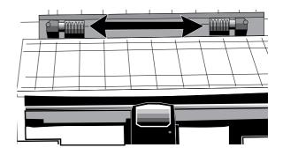
5. Place the first two holes in the paper over the tractor pins 7. on either side and close the tractor covers.
