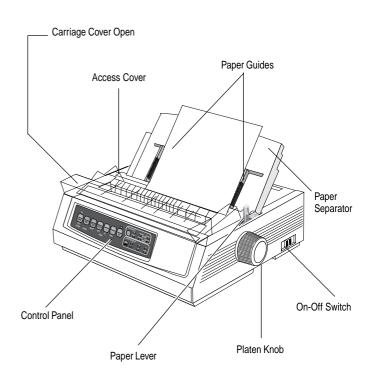
Set up for Rear Feed of Continuous Forms
