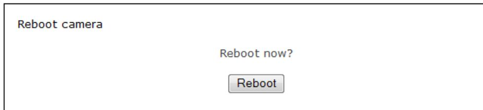
Click Reboot to restart the Y-cam. Rebooting the camera will retain all the settings and configurations.
