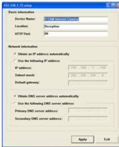
4. Enter a unique name for the camera, the location (optional) and leave the default port number as 80. “Obtain an IP address automatically” and “Obtain DNS server address automatically” are selected by default, if you are confident enough to enter your own settings, you can do so by selecting “Use the following IP address” and follow the guidelines on the next page.
